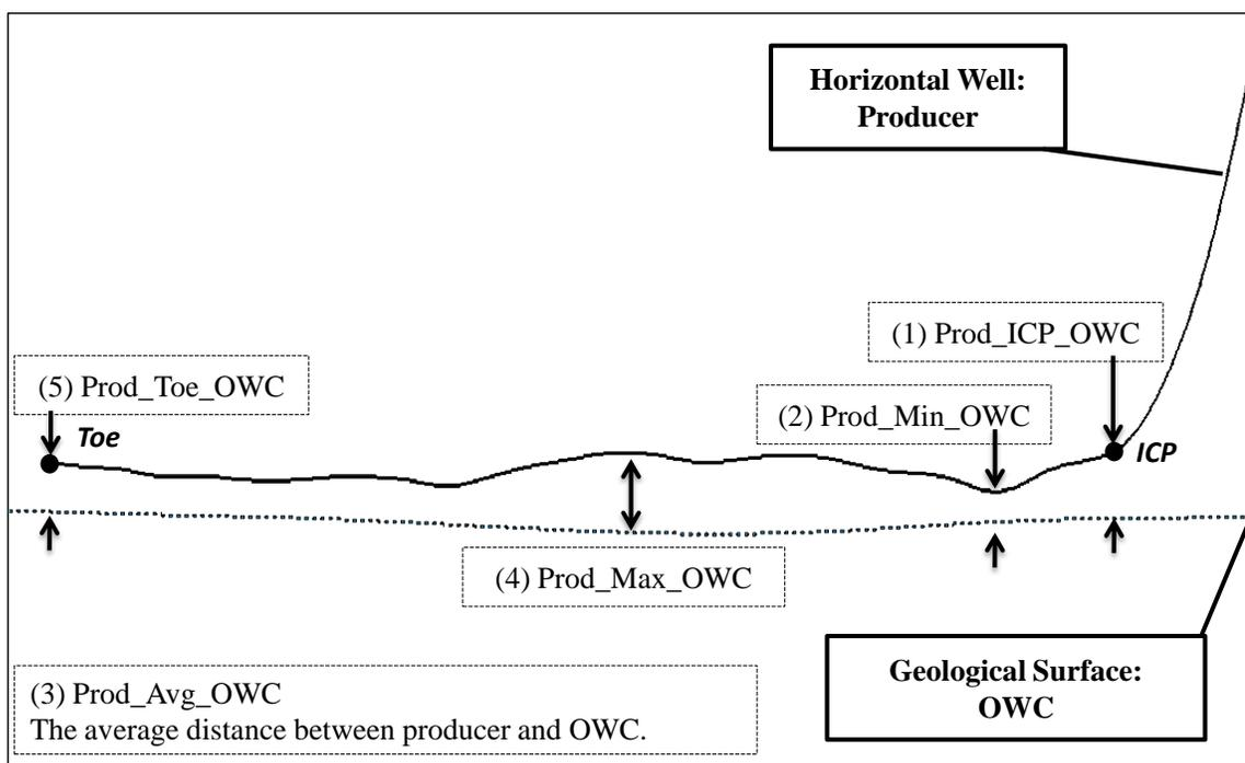
**Figure 4–1 Five Well placement attributes from a horizontal producer and the Oil-Water-Contact (OWC) geological surface**
