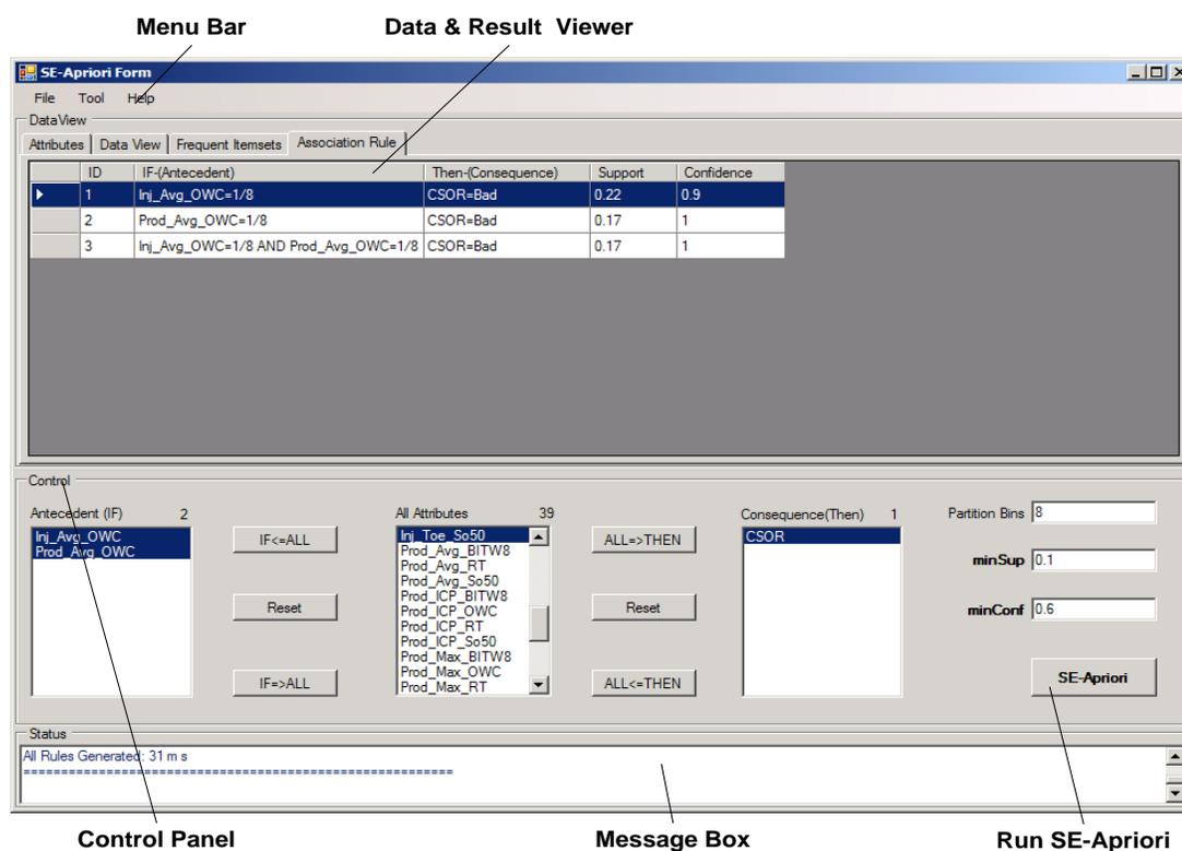
**Figure 4–10 The graphical user interface of the SE-Apriori tool**
