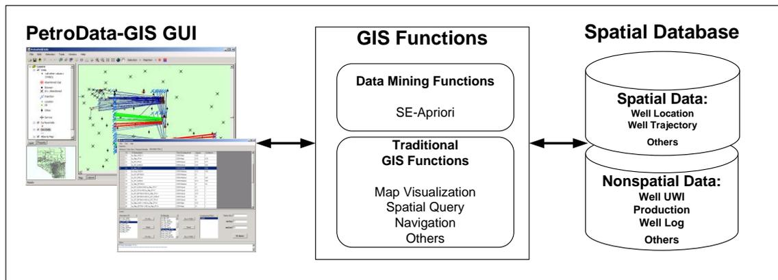
**Figure 4–7 Architecture of the PetroData-GIS prototype**
