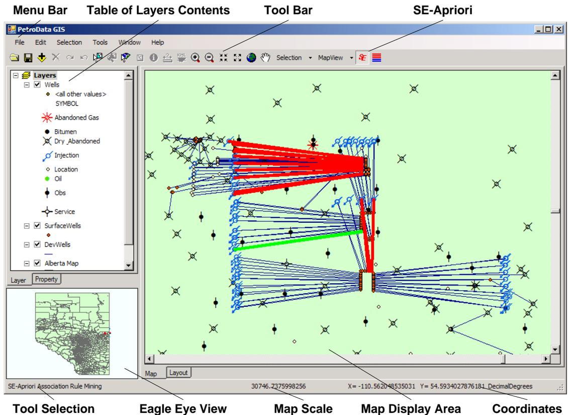
**Figure 4–9 The main graphical user interface of PetroData-GIS prototype**
