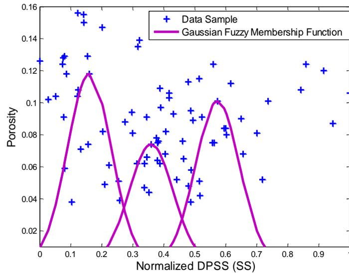
**Figure 3–6** Gaussian fuzzy membership functions in the DPSS-Porosity space
