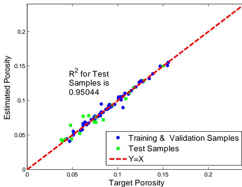
**Figure 3–19** Cross plot of estimated and core porosity values
