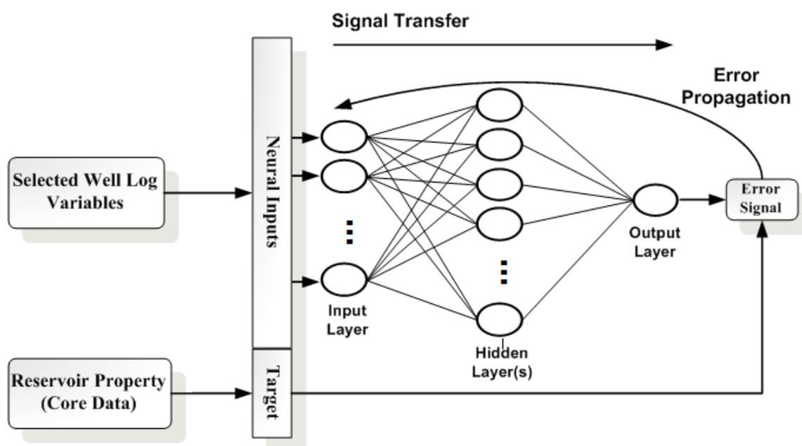
**Figure 3–9 The Multilayer Perceptron (MLP) model in the pattern recognition step for reservoir characterization**
