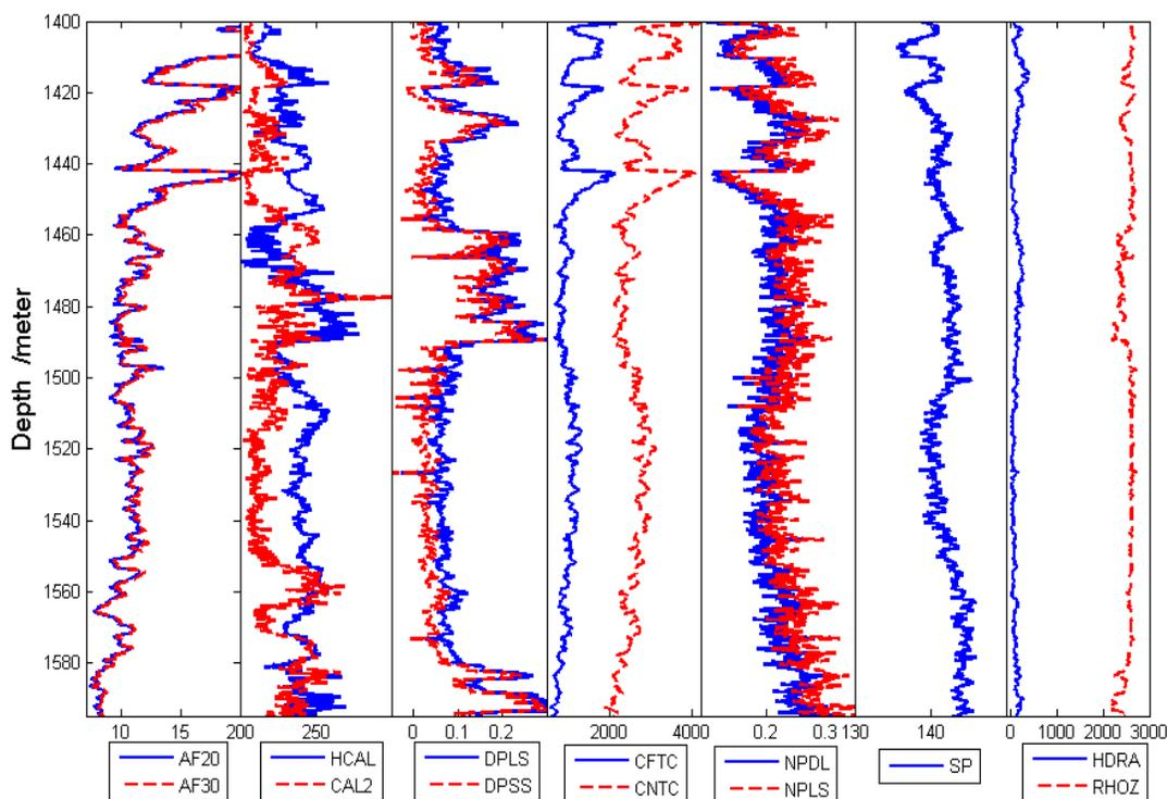
**Figure 3–17 Well log variables versus depth.**
