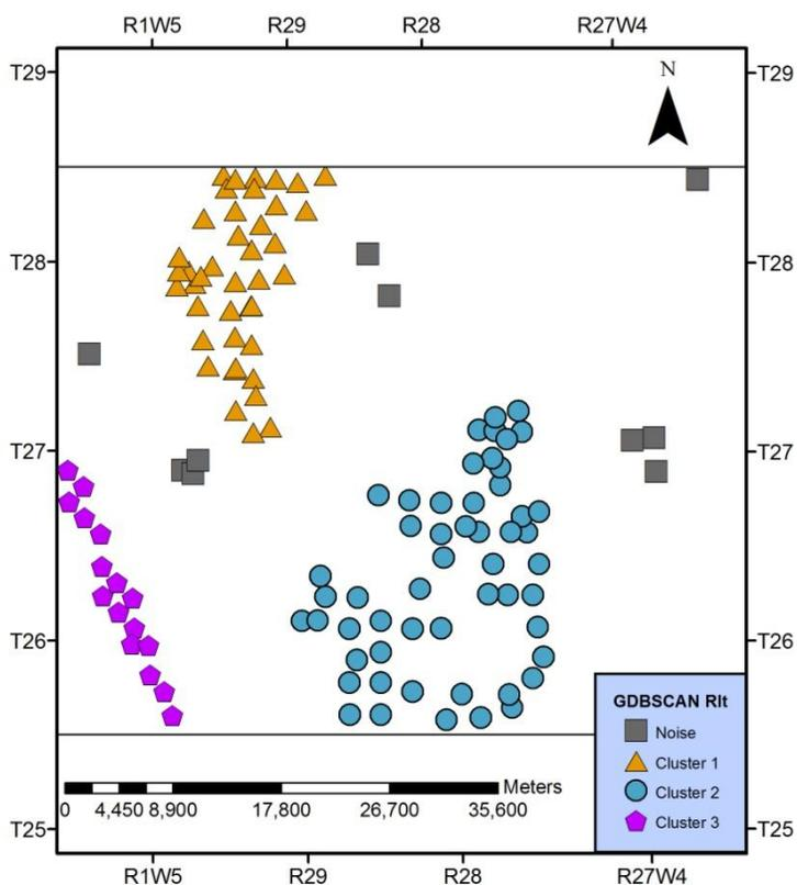
**Figure 3–14 Clustering results from GDBSCAN over core analysis data**
