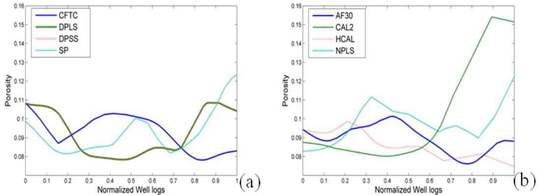
**Figure 3–16 Fuzzy curves for partial well log variables: (a)AF30, CAL2, HCAL, NPLS (b)CFTC, DPLS, DPSS, SP.**
