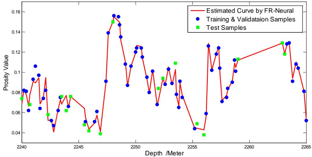
**Figure 3–18** Estimated and core porosity values from MLP with depth
