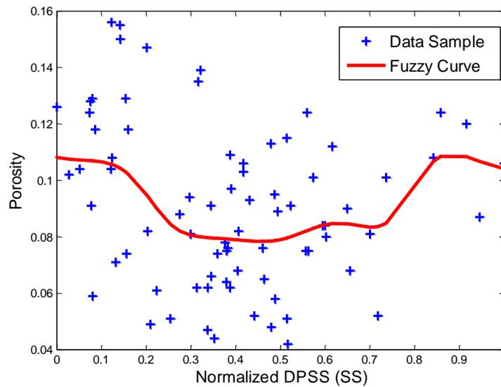
**Figure 3–7** Fuzzy curve of DPSS to porosity
